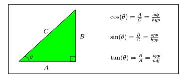
In the picture above we assume that A, B, C > 0 and we have drawn the triangle so that  $0 < \theta < \pi/2$ , it is an *acute* angle. You may recall that the side A is **adjacent** to the angle  $\theta$  while the side B is **opposite** the angle  $\theta$ . The longest side C is called the **hypotenuse**. We know the **Pythagorean Theorem** states  $A^2 + B^2 = C^2$ .
