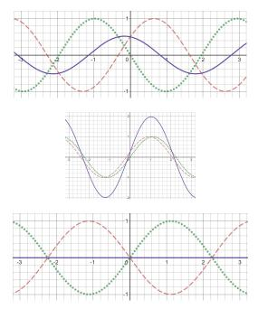
The picture above illustrates **destructive interference**. In all the cases above we are adding waves with the same frequency, only the phase differs.
