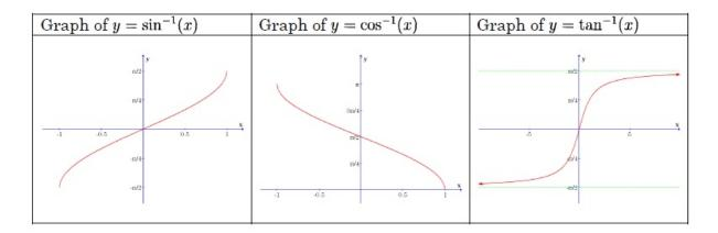
The green lines illustrate horizontal asymptotes of inverse tangent. The occur at  $y=\pi/2$  and  $y=-\pi/2$ . These are all local inverses, this is the reason the "inverse tangent" failed to provide us the correct angle outside quadrants I and IV. The inverse tangent function is only truly the inverse of tangent in quadrants I and IV for  $-\pi/2 < \theta < \pi/2$ .
