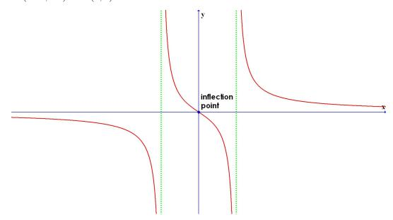
One physical interpretation mathematics found in the previous example is that y = f(x) could be a graph of the electric potential along the x-axis for two positive point charges placed at x = -2 and x = 2. A divergence in the potential signals the presence of localized charge.
