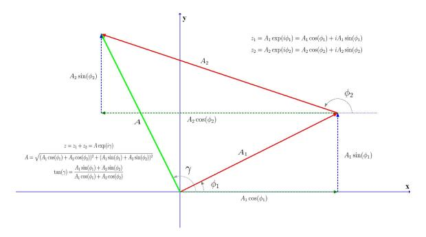
If you had highschool physics you should recognize the construction above as the so-called "tip-2-tail" method of vector addition. Have no fear, it's just trigonometry. Moreover, it is no hard to see the calculation above easily generalizes to three or more vectors.
