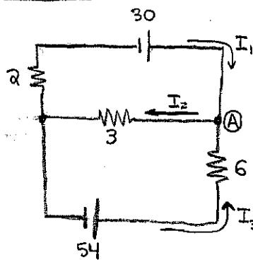
$$\text{top loop : } 2I_1 - 30 + 3I_2 = 0 : \mathcal{E}_q^{\text{up}} \quad \textcircled{I}$$
