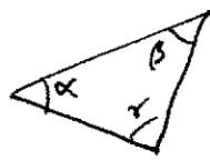
$$\begin{aligned}\alpha + \beta + \gamma &= \pi \\ \alpha + \beta &= \pi - \gamma \\ \sin(\alpha + \beta) &= \sin(\pi - \gamma) \\ &= \sin \pi \cos \gamma - \cos \pi \sin \gamma \\ &= \underline{\sin \gamma} \quad //\end{aligned}$$
